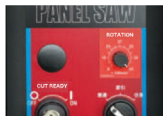
Inverter for saw rotation
