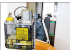
Saw carriage auto lubrication
